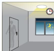
3 After elapse of hold time, the sensor dims the light at a low light level if no new motion trigger.
