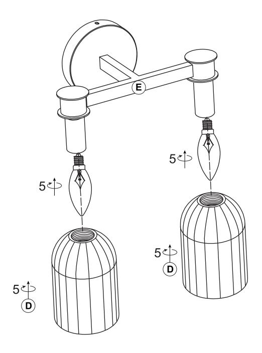
Install a light bulb (not included) on the sockets.
