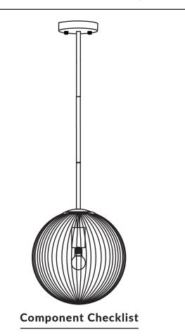
REF Α В C D Ε F G Н **PART** Ribbed Expansion Tubes Mounting Nut Brass **Brass** Lamp Screws NAME Clear Bracket Lock Canopy Rod Holder Glass Ball QTY 1 4 4 2 1 1 1 1
