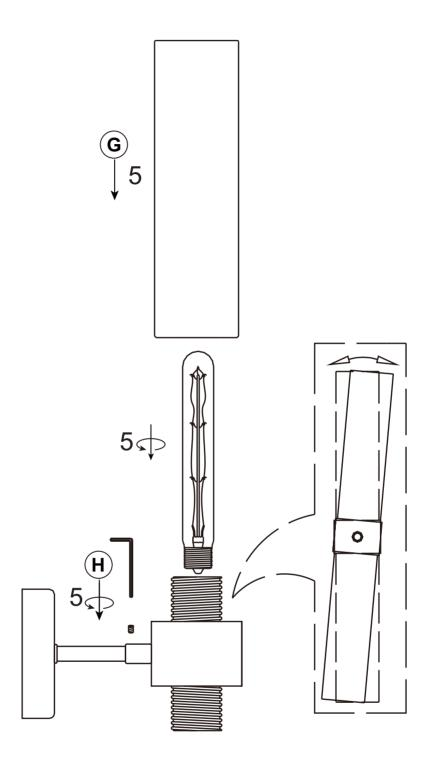
Install a light bulb (not included) on the sockets.
