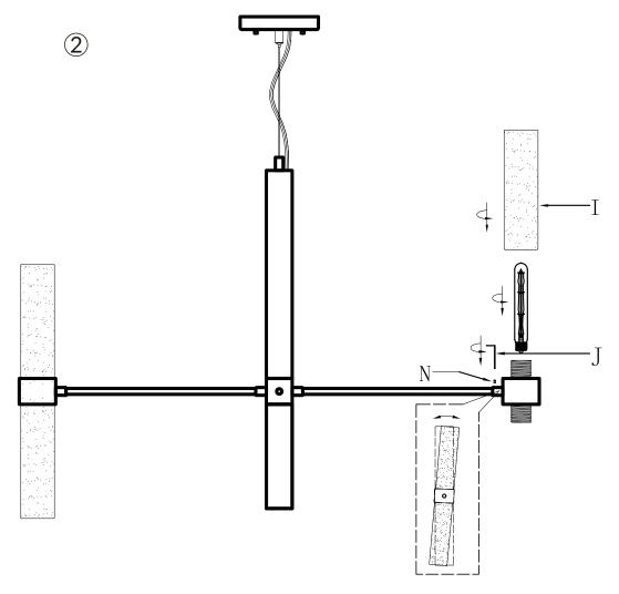
•Install the bulbs (NOT INCLUDING) on the sockets, and then attach the glass pipes (I) on the sockets. (CAUTION: YOU CAN USE THE HEX WRENCH TO ADJUST THE KIMI SCREWS IN THE ARMS VERTICALLY ACCORDING TO THE ILLUSTRATIOIN IF YOU FIND THE ARMS NOT SO VERTICAL. AND PLEASE DO NOT ADJUST THE ARMS VERTICALLY THROGH THE GLASS PIPES(I))
