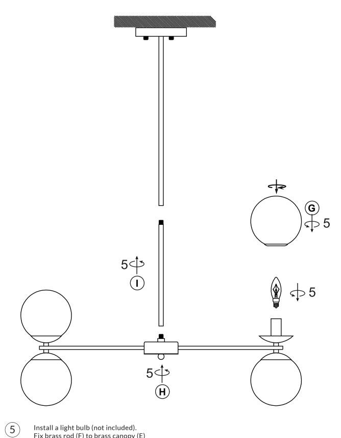
Install a light bulb (not included). Fix brass rod (F) to brass canopy (E) Fix lamp body (H) to brass rod (F). Fix glass balls (G) to lamp body (H), as shown.
