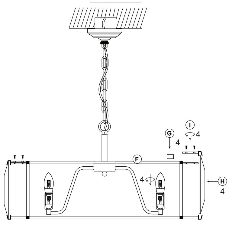
Insert the alabaster flakes (H) to lamp body (F) slot and lock it with screw sets (I). Attach magnet (G) to lamp body (F). Install bulbs (not included) to lamp body (F), as shown.
