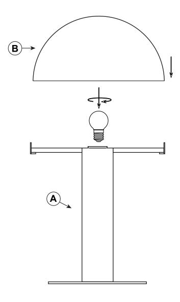
Insert E27 globe into lamp holder screwing in until they are firm. (globe not included).
