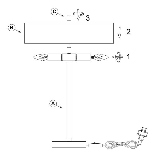
Insert E14 globes into each lamp holder screwing in until they are firm. (globes not included).
