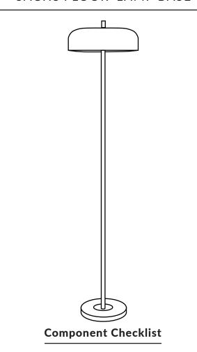
REF Α В C D Ε F G **PART** Double Bulb Top Pole NAME Lamp Base Lower Pole Middle Pole Head Finial Socket QTY 1 1 1 1 1 1 1
