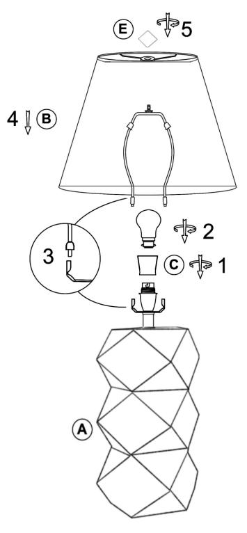
Carefully unpack all parts from box and place lamp base on flat surface. Screw lamp holder skirt on to lamp base (A).
